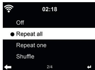
Select the playback mode of media center – Off (no repeat or shuffle), Repeat all, Repeat one, or Shuffle.
