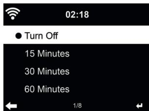
Turn off or set the sleep time to 15/30/60/90/120/150/180 minutes. Once the time is set, there will be a bed icon with remaining minutes at the top right corner. The DR 470 will shut down once the time runs out. Press Sleep on the remote control for the shortcut of this function.
