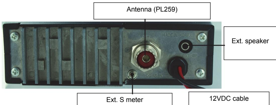
Connect your CB antenna via PL connector to the 50 Ohms antenna jack at the rear of your AE 6891. For best range the antenna must be adjusted for CB radio. Use a standing wave meter to check and to adjust the antenna. Adjust the antenna for best standing wave ratio on a medium channel. If you are using 80 channels optimize on channel 1, for 40 channels on channel 20 and for truckers we generally recommend channel 9.
