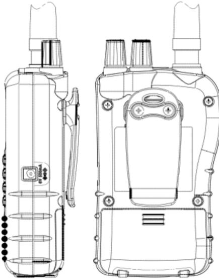
To make your scanner easier to carry when you are on the go, use the supplied belt clip. Use a Phillips screwdriver and the supplied screws to attach the clip to the scanner.
