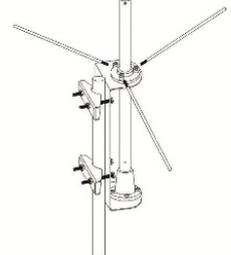
7. Tighten the crews to fix the position, then screw the 3 rods as the drawing.
