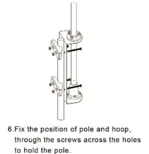
6. Fix the position of pole and hoop, through the screws across the holes to hold the pole.
