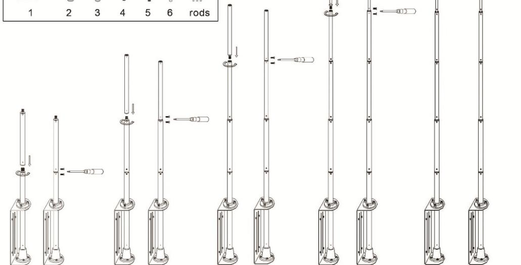
1. Rotate the base part and the 2nd whip, tighten the crew.
