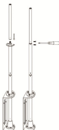
2. Rotate the 3rd whip to the 2nd whip, tighten the crew.
