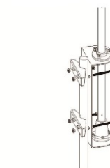
6. Fix the position of pole and hoop, through the screws across the holes to hold the pole.
