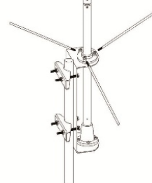
7. Tighten the crews to fix the position, then screw the 3 rods as the drawing.
