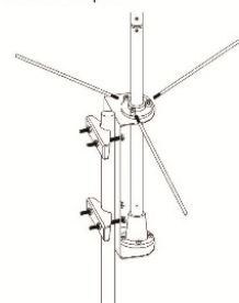
7. Tighten the crews to fix the position, then screw the 3 rods as the drawing.
