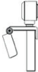
Attach the camera mount to the top edge of your monitor by pressing the bottom of the mount against the back of the screen.
