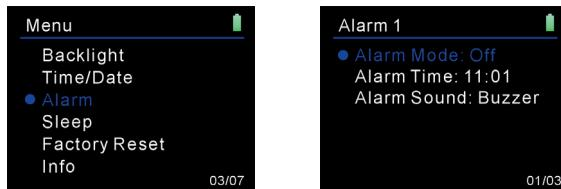
Rotate the <TUNING /SELECT> control to choose setting up Alarm 1 or Alarm 2. Press the <TUNING /SELECT> control to enter the detailed settings.
