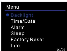
Select the illumination **Level** of the backlight (High/Medium/Low) and the duration of **Timeout** (On/10/20/30/45/60/90/120/180 sec). By setting a time for the Timeout, the display will automatically dim down if no operation is done during the selected period of time.
