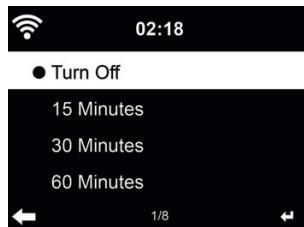
Turn off or set the sleep time to 15/30/60/90/120/150/180 minutes. Once the time is set, there will be a bed icon with remaining minutes at the top right corner. The DR 883 will shut down once the time runs out. Press Sleep on the remote control for the shortcut of this function.
