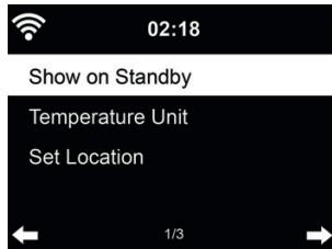
DR 883 is able to display current weather information (refer to 16.1) under standby mode. Turn on Standby Display and set Temperature Unit (°C or °F) to get the weather displayed at the standby mode.
