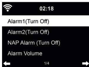
There are three independent alarms - 2 alarms of absolute time setting (**Alarm 1** and **Alarm 2**) and 1 alarm for relative time setting (**NAP Alarm**). Press **Alarm** on the remote control to enter this menu directly.
