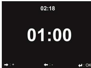
Press **◀/▶** to set the timer, press **OK** to start. The timer will count down and beep sound when it reaches 00:00. To cancel the timer, enter the timer screen and press **OK** again.
