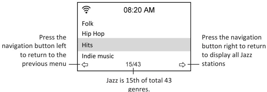
3. Press the right navigation button to display all jazz stations available. Highlight a station and press the enter button to connect to the station.
