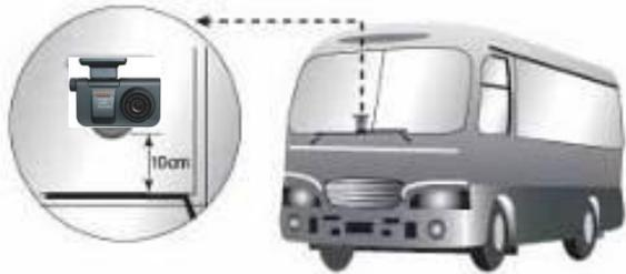
4. Truck : Attach the bracket on the center of the front windshield about 10cm above the wipers and arrange the cables neatly with the provided wire splice clips so as not to disturb the field of vision of the driver.
