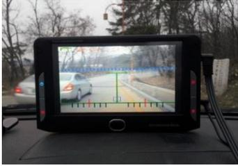
**10.** When the "Red" and "Blue" LEDs are turned on and the image in front of the car appears on the monitor, basic installation of K11 is completed.
