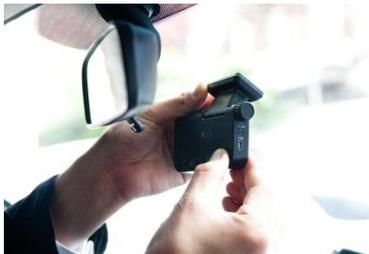
**4.** With the angle adjusting bolt, temporarily and lightly fix K11 vertically from the side view.
