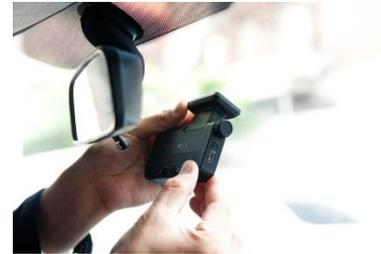
**3.** Insert K11 to the bracket and make sure it is vertical from the side view by using the angle adjusting bolt.
