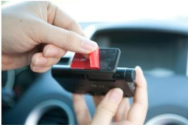
**2.** Attach the bracket firmly to the front windshield behind the rear view mirror maintaining the bracket's balance.
