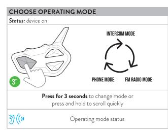
Note: By pressing simultaneously Vol + and Vol - for 1 second, BT Rush communicates the selected mode.
