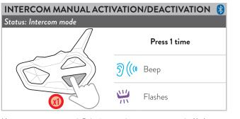
**Note:** to communicate with Rider 1 repeat the process pressing the **Up button.**
