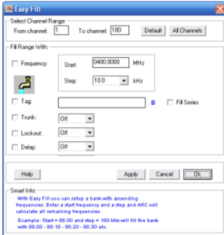
In the top frame the channel range is selected. DEFAULT will set the start and end channel of the selected bank.
