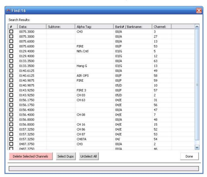
The results are sorted by frequency. You can delete duplicates by ticking the box in front of the frequency. Select Dups automatically selects the duplicate frequencies.
